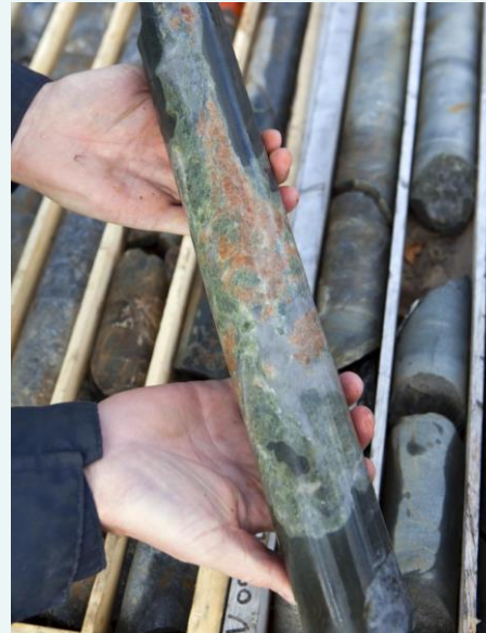
Calc-silicate alteration in amphibolite
