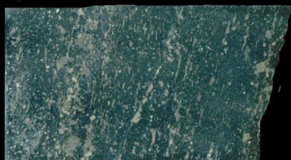
strong chlorite-garnet-magnetite alteration
