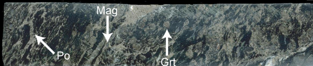
strong chlorite-garnet-magnetite-sulphide alteration
