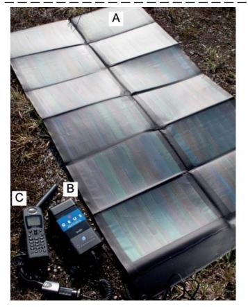
Figure 2. Equipment used for charging the digital field data capture system: a) solar panels (62W P3 Powerpack from Select Solar Ltd.) were used to generate power; b) an external battery (myPower ALL Plus MP3750 from Tekkeon, Inc.) was charged by the solar panel; c) charging an external device, in this example a satellite phone.
