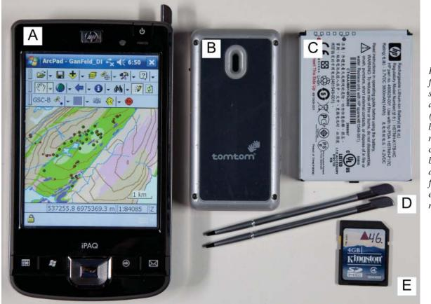
Figure 1. The digital field data capture system consists of: a) HP iPAQ PDA (310  $\in$ ); b) wireless GPS receiver (48  $\in$ ); c) HP extended battery (59  $\in$ ); d) PDA stylus (7  $\in$ for each stylus); e) secure digital (SD memory card (15  $\in$ ).
